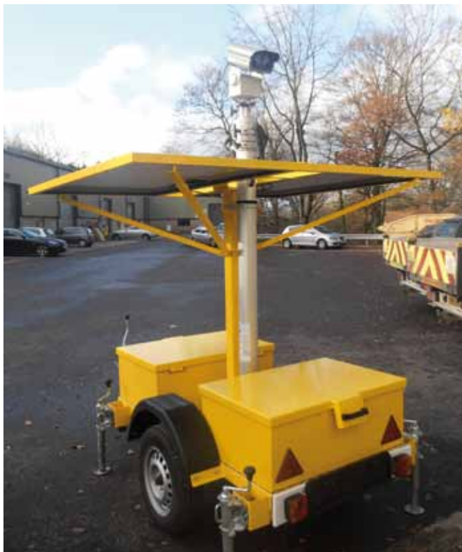
MVIS’ Solar 2012 multi-use trailer platform – an integral part of its new Portable Solar Powered Journey Time Solution
