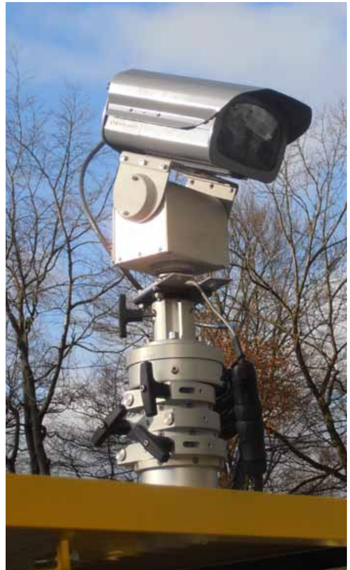
The M4/5 temporary ITS solution featured Vysionics' SkyHawk integrated ANPR cameras along with MVIS' VMS-Cs and Web Studio sign management and control system
